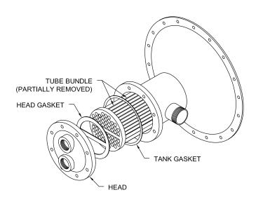
4. When replacing the heat exchanger head, use a torque wrench to tighten the bolts/studs and nuts. Use the following chart as a guide. All torque values apply to well-lubricated nut bearing surfaces.
